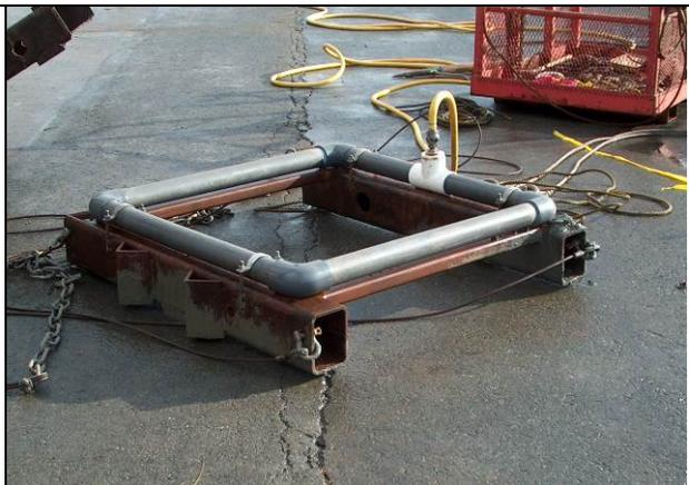
**Figure I.5-1b Simple Air Bubble Curtain System Used to Attenuate Noise**
