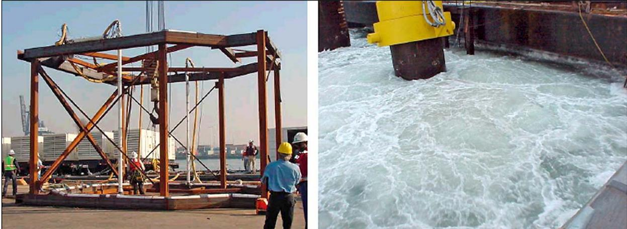
**Figure 2-22. Dual-Stage Unconfined Air Bubble Curtain**
