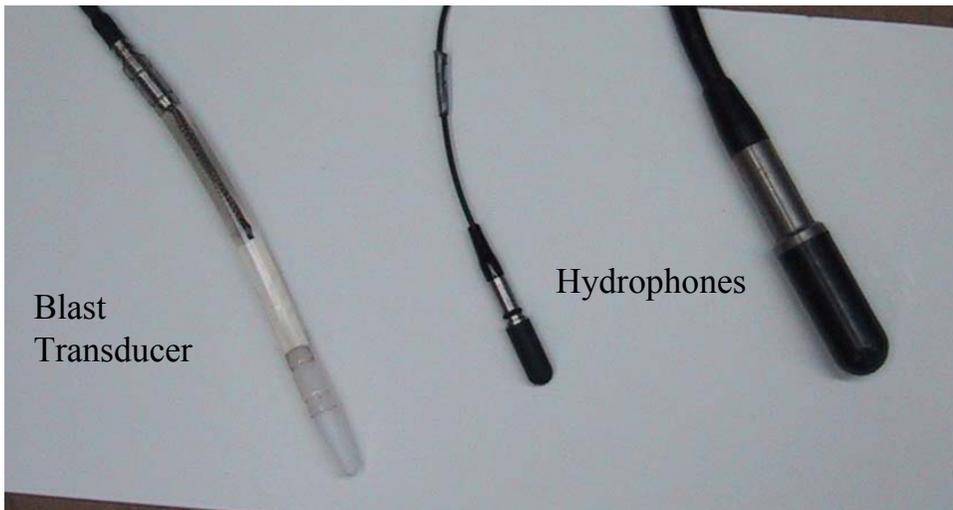
**Figure II-5. Example of Different Pressure Sensors**
