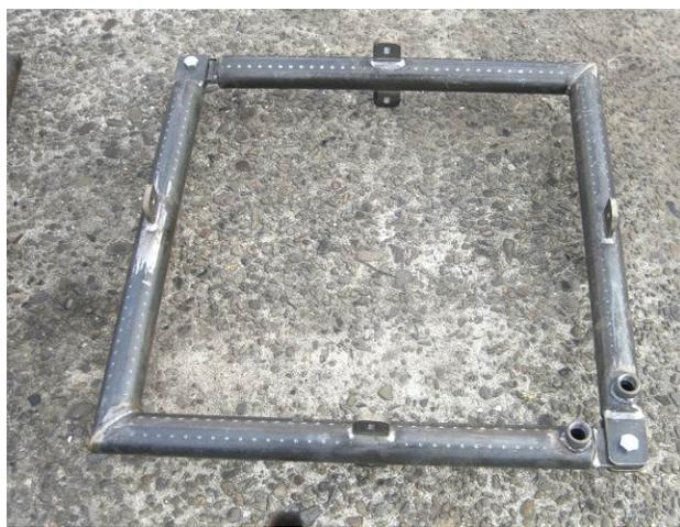
**Figure I.3-31 One Level of the Multi-Stage Bubble Ring—Tongue Point Facility Pier**
