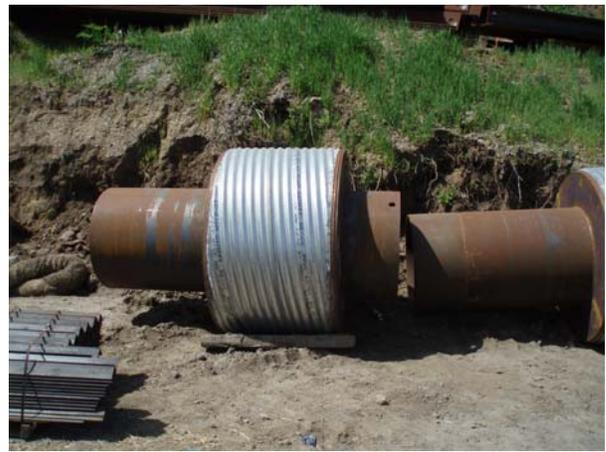
**Figure I.13-3b Shallow Water Isolation Casing**
