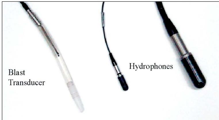
Figure 2-17. Pressure Sensors
