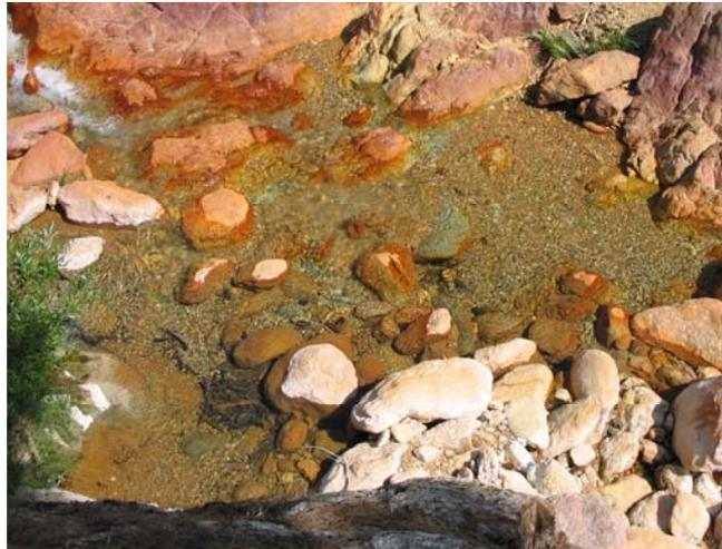
Channel margin bed material detail at bedrock cascade nr LP STA 3+00, Little Backbone Creek, July 31, 2003. Note median grain size is approximately 3 mm and deposit is minimally embedded.
