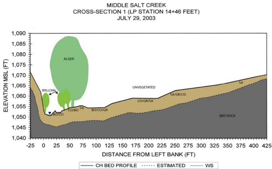
**Figure 3-41 Middle Salt Creek Cross Section #3**
