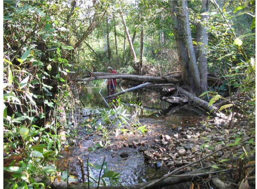
View upstream from mid-channel nr LP STA 10+25 ft to woody debris influenced pool at LP STA 10+56 ft, Salt Creek, October 5, 2003. Note that the maximum pool depth was 3.03 ft.
