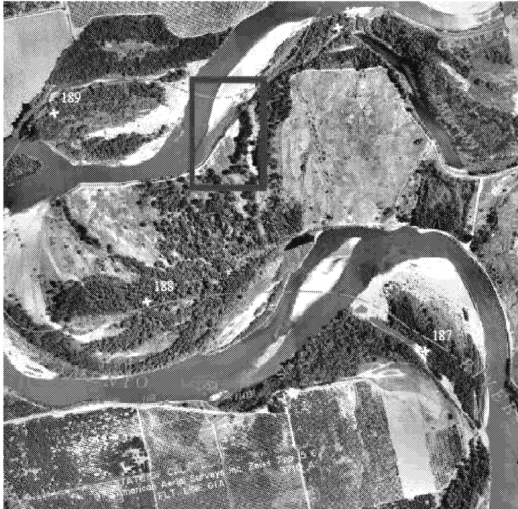
Figure 2. Example of a scour channel that forms on the downstream end of a point bar, providing seasonally inundated, shallow-water habitat that can support rearing of salmonid fry. (Photo Source: CDWR 1999)
