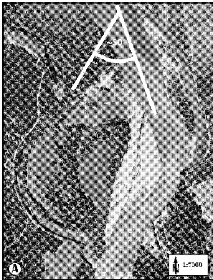
Figure 57. (A) Aerial photo of La Barranca near river mile 237 taken in 2004. The diversion angle and the core location are shown within the photo. (B) Granulometric profile for core LBCOR1.
